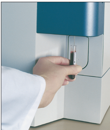
Fig. 5: In the XS-800i, blood samples can only be analysed manually and in open condition which is advantageous especially for minimal blood volumes.
